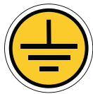
Central earthing point
