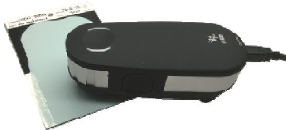
The search is based on the measured  $L^*a^*b^*$  - values and a list with nearest recipes will be shown together with the colour difference.
