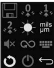
**Memory Mode:** Turns Memory Mode ON. The gage will store and maintain a running average for up to 999 readings. Stored measurements can be downloaded to PosiSoft Desktop Software (pg. 10). When **Memory Mode** is ON, the following menu options appear:
