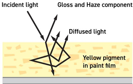
The Novo-Gloss 20/60/85 version with haze compensates for reflection from within the coating for highly reflective pigments, metallic coatings and speciality pigments, allowing the haze of any painted surface to be measured.
