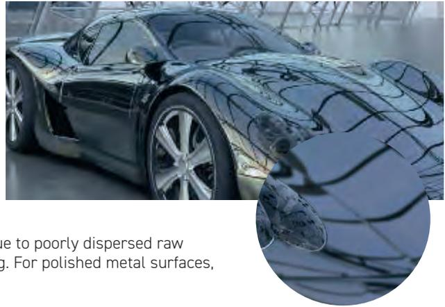
In the coatings industry, this microscopic surface texture is often due to poorly dispersed raw materials, incompatible raw materials or oxidation and weathering. For polished metal surfaces, haze is often associated with polishing marks or chemical residue.
