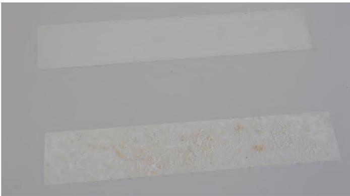
Clear tape is pressed on the measurement surface, torn away and stuck onto white paper - For reference a clean piece of tape is also stuck on the same white paper.
