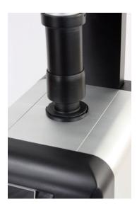
Take a reading on the checking standard by pressing the tick icon and compare the result with its assigned value. The value must match the assigned value within the tolerances printed on the label.
