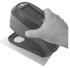
3. Press the instrument firmly to the shoe and hold steady until the display indicates that the measurement is complete.
