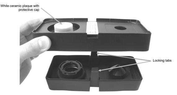
3. After cleaning, align the two arrows on the end before reassembling the sections. **Note:** The tabs will not lock correctly if assembled in the opposite direction.
