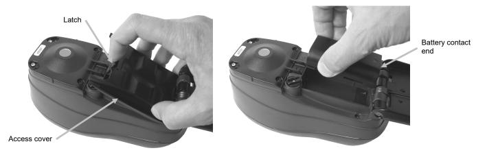
5. Reinstall the battery access cover by inserting the back edge first and then pressing downward until the access cover locks into position.
