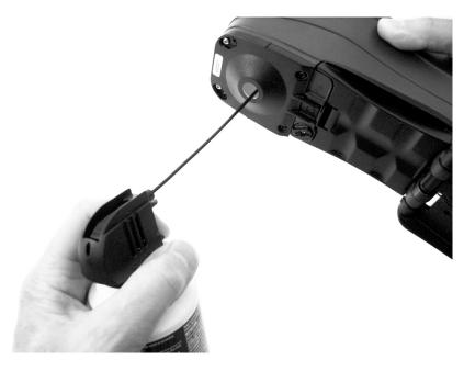
**IMPORTANT:** If can air is used for cleaning, do not invert or tilt the can during use. This could cause damage to the optics.
