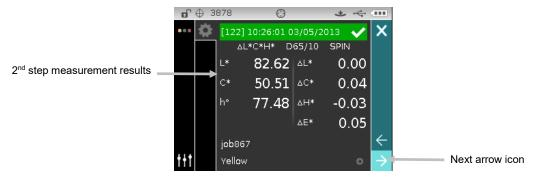
7. Position the instrument on the sample as described on the screen and take the measurement.
