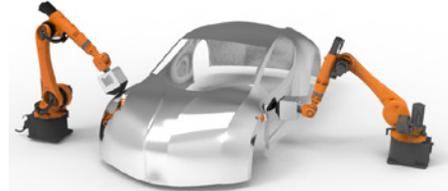
TAMS measurement sensor integrates fully into an inline inspection process and is designed for top coat evaluation as part of the production line or offline measurement cell. The sensor is able to capture high resolution maps of surfaces and has the possibility to measure e-coat and raw materials.
