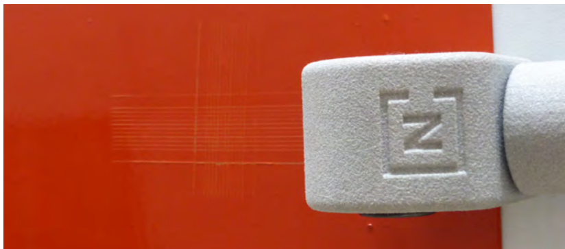
ASTM Class 0, ISO Class 5, Undamaged area: 16.5%
